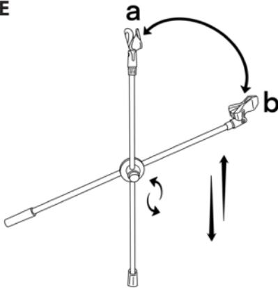
Loosen the other screw(6),to adjust the height of retaining rod(5).
